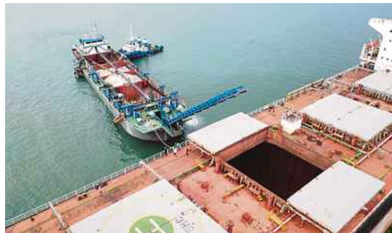
A vessel transporting and loading marine sand onto a mother vessel for export or to reclamation sites.
